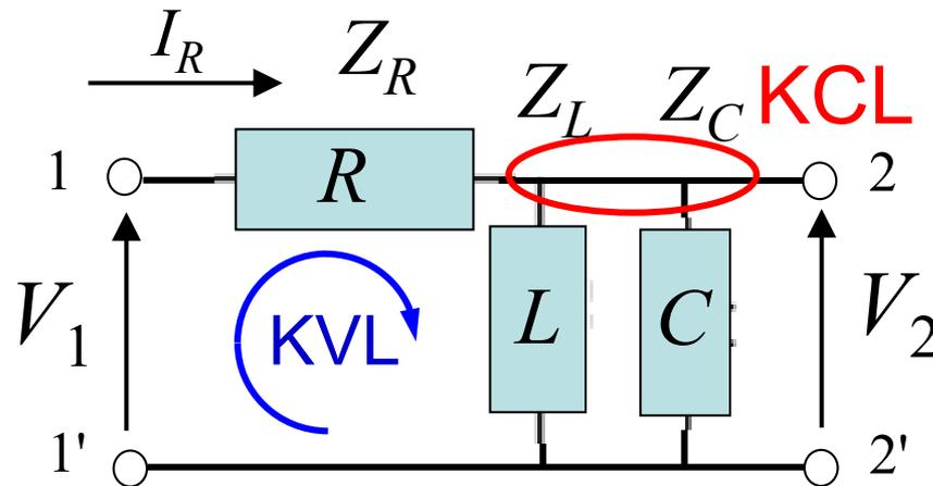
$$V_2 = V_1 - I_R Z_R = V_1 - \frac{V_1}{Z_R + 1 / \left( \frac{1}{Z_L} + \frac{1}{Z_C} \right)} Z_R$$
